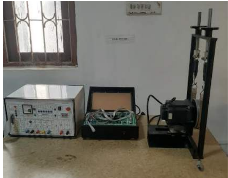
SRM Drive System with Loading Setup
