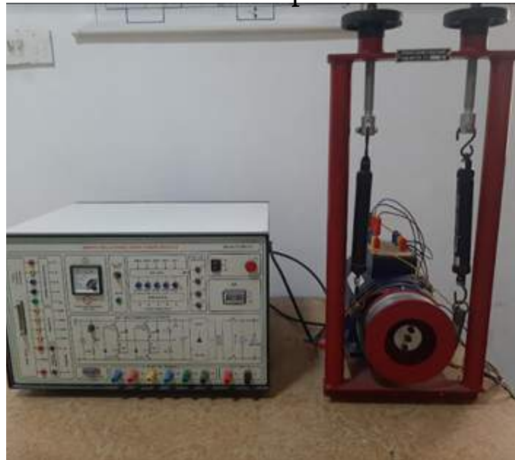
SRM Drive System with Loading Setup
